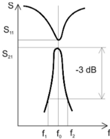
Figure 4: Resonant curve.
