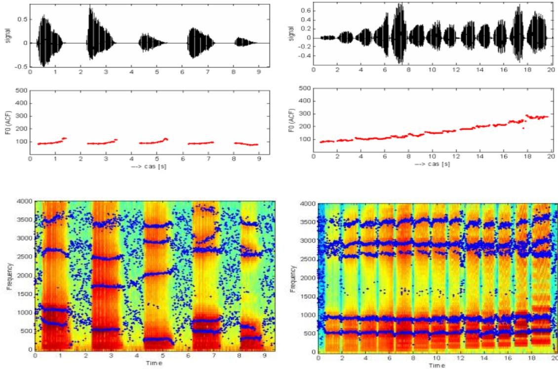
Figure 2: The left column displays the Czech vowels; in the right column there is the singing vowel /a/ (in a musical scale). The waveforms in time domain are in upper figures; the results of the fundamental frequency detection using algorithm based on autocorrelation function are in the middle figure and the results of formant detection using LPC are in the bottom.
