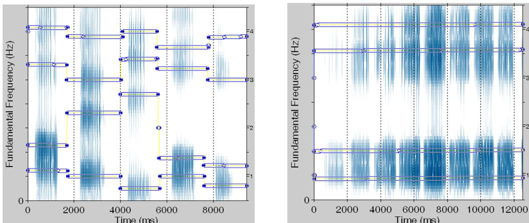
Figure 3: Left: formant tracks for Czech vowel synthesis; right: formant tracks for /a/ in musical scale
