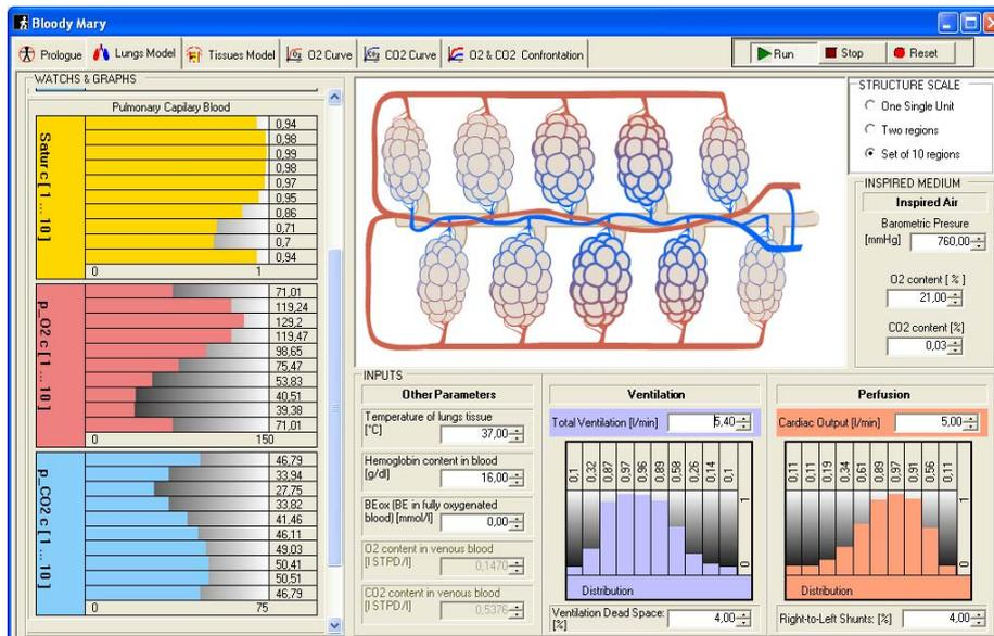
**Fig. 4.** An example of a simulator user interface combining custom MS .NET controls (bar graphs) with Flash animations (alveoli)
