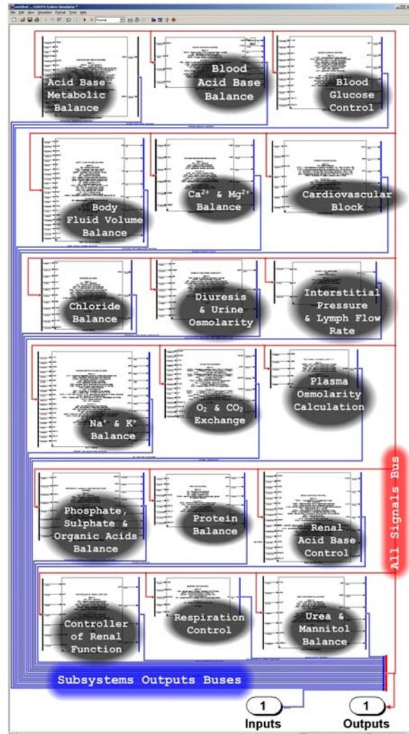
Fig. 2. The inner structure of simulation chip from fig. 1. The structure looks like an electronic circuit with interconnected chips, that are represented by simulation chips of a lower hierarchical level. Interconnected simulation chips depict the core structure of the large-scale model of physiological regulations
